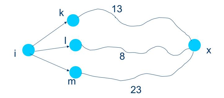
The message will be sent from i to I as the cost of the path to x is minimum through I
