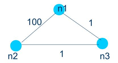
•However, when the link n1-n3 is broken, this will be noted by n1 in its routing table.
