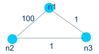
•Suppose each node broadcasts its routing table stamped with an increasing sequence number.
