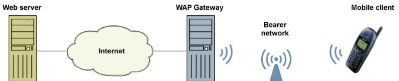
The WAP gateway carries out the necessary protocol translation and content encoding
